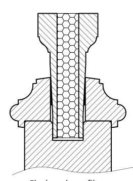
Flush sash profile with moulding
