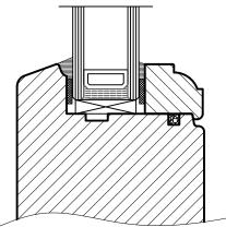
Rebated sash profile with Ovolo glazing bead
