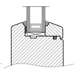
Rebated sash profile with Splayed glazing bead
